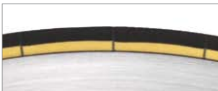
Vitrified CBN grinding tool with neutral zone.
